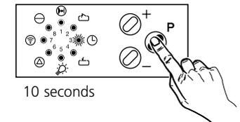
If an automatic timer is used, an external photocell to monitor the through-traffic area must be connected and activated in accordance with pt 22/1 (Earlyclosing after driving past the through-traffic photocell). Otherwise no automatic timer function is possible.
