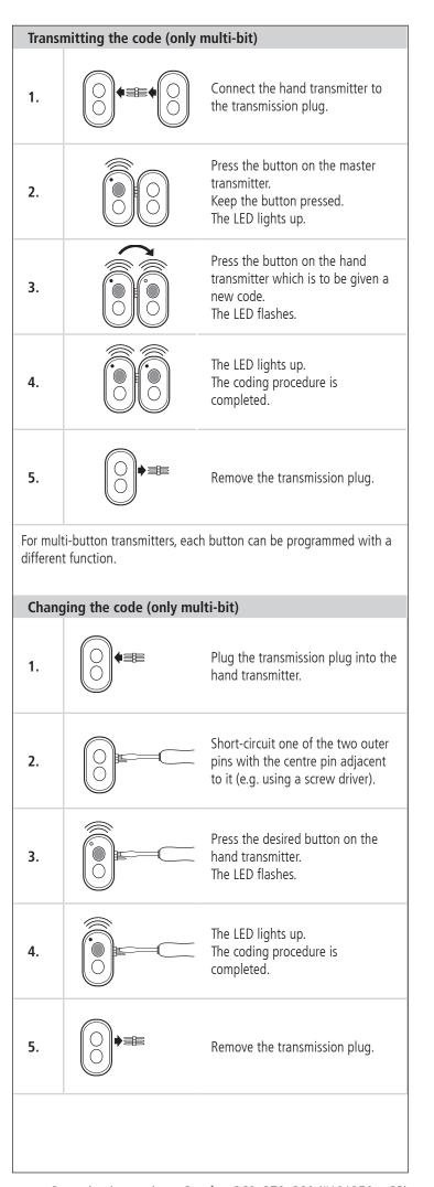
After the hand transmitter has been re-coded, the operator system must also be re-programmed to respond to the new code. For multi-channel transmitters, the programming process must be carried out for each button separately.
